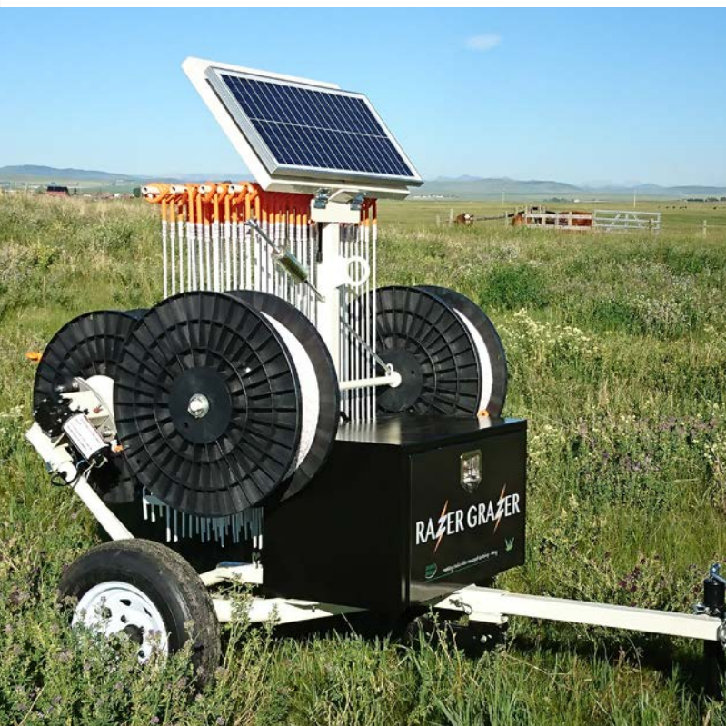
This commercially available solar trailer system by Range Ward can quickly deploy electric fence for flexible forage management. Credit: Norm Ward, Range Ward.
